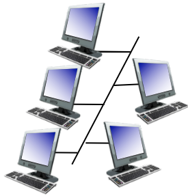
shared wire (e.g., cabled Ethernet)
