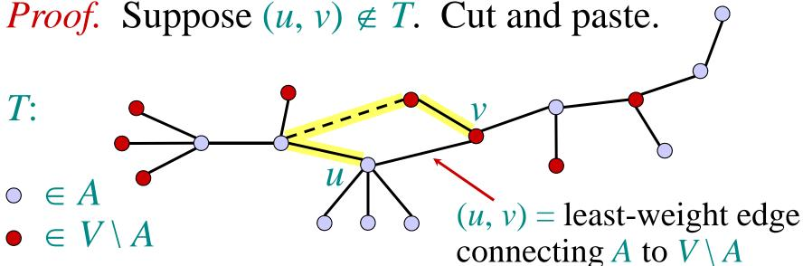
Consider the unique simple path from u to v in T. Swap (u, v) with the first edge on this path that connects a vertex in A to a vertex in  $V \setminus A$ .
