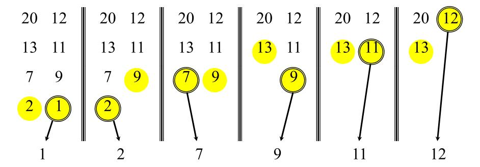
Time  $dn \in \Theta(n)$  to merge a total of n elements (linear time).
