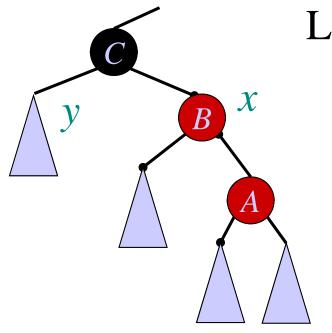
p[x] = right[p[p[x]]] y = left[p[p[x]]] color[y] = BLACKx = right[p[x]] LEFT-ROTATE(C)
