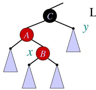
p[x] = left[p[p[x]]] y = right[p[p[x]]] color[y] = BLACKx = right[p[x]] LEFT-ROTATE(A)
