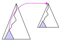
**Idea:** In primary 1D range tree of *x*-coordinate, **every** node stores a **secondary** 1D range tree based on *y*-coordinate for all points in the subtree of the node. Recursively search within each.
